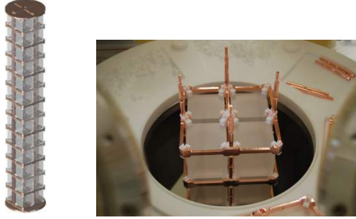
Figure 3.9: CUORE-0 tower rendering and close up. Left: the 52 \times 5 \times 5 \text{ cm}^3 \text{TeO}_2 crystals of 750 g each are disposed in 13 floors in groups of 4, for a total mass of 39 kg. The tower skeleton is made by ultra clean copper and the crystals are plugged to the frames by PTFE clamps. Right: close up of the tower during the assembly; crystals, copper structure and PTFE brackets (white components) are visible.
