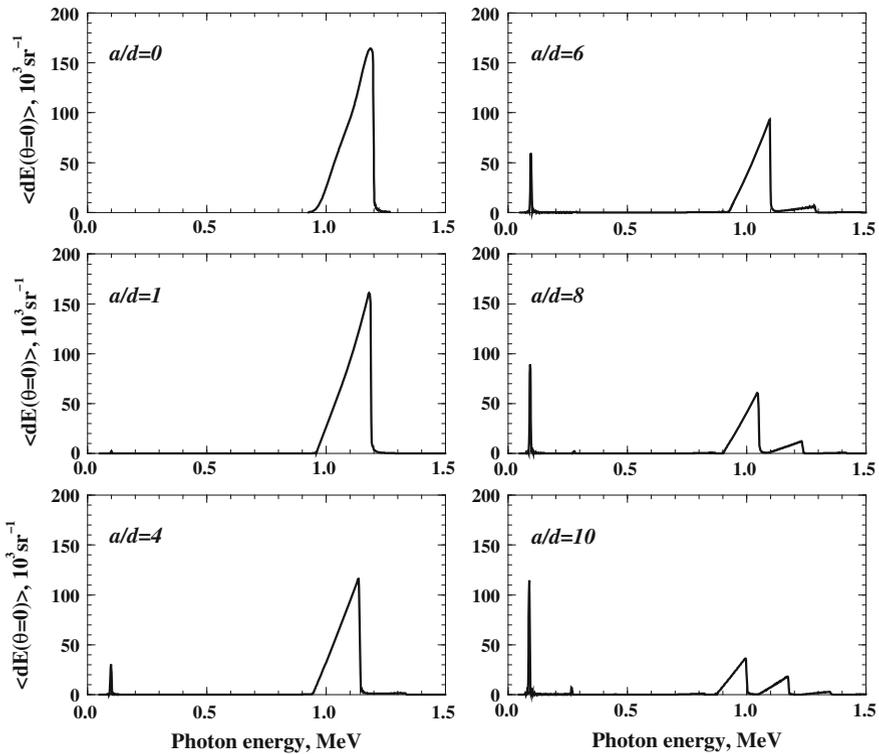
**Fig. 2** Spectral distribution of the total radiation emitted in the forward direction ( $\vartheta = 0^\circ$ ) for  $\varepsilon = 0.5\text{ GeV}$  positron channeling in Si (110) crystallographic plane calculated at different  $a/d$  ratios. Other parameters are given in the text
