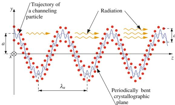
**Fig. 1** Schematic representation of the crystalline undulator. *Closed circles* mark the atoms belonging to two neighbouring crystallographic planes (separated by the interplanar distance  $d$ ) which are periodically bent with period  $\lambda_u$  and amplitude  $a$  (the  $y$ - and  $z$ -scales are incompatible!). *Thin solid line* illustrates the trajectory of the particle, which propagates along the centerline (the undulator motion) and, simultaneously, undergoes channeling oscillations
