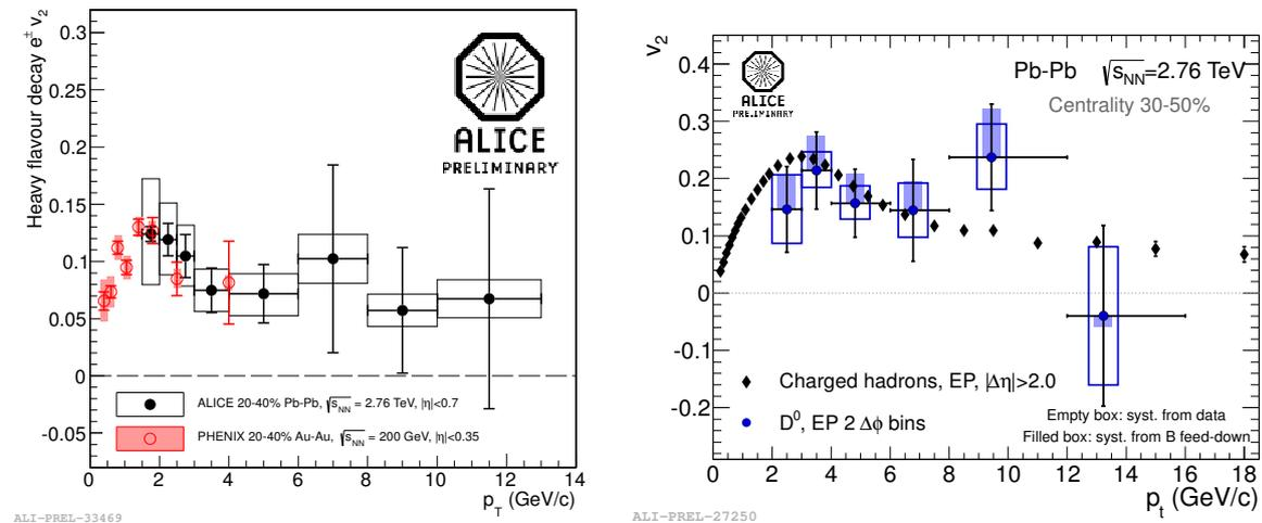
**Figure 4.** Elliptic flow of open heavy-flavour at RHIC and LHC. Left:  $v_2$  of heavy-flavour decay electrons, measured by ALICE [23] and compared with the same measurement by PHENIX at RHIC [13]. Right:  $D^0$  meson  $v_2$  as a function of  $p_T$ , measured by ALICE and compared with charged hadrons [23].
