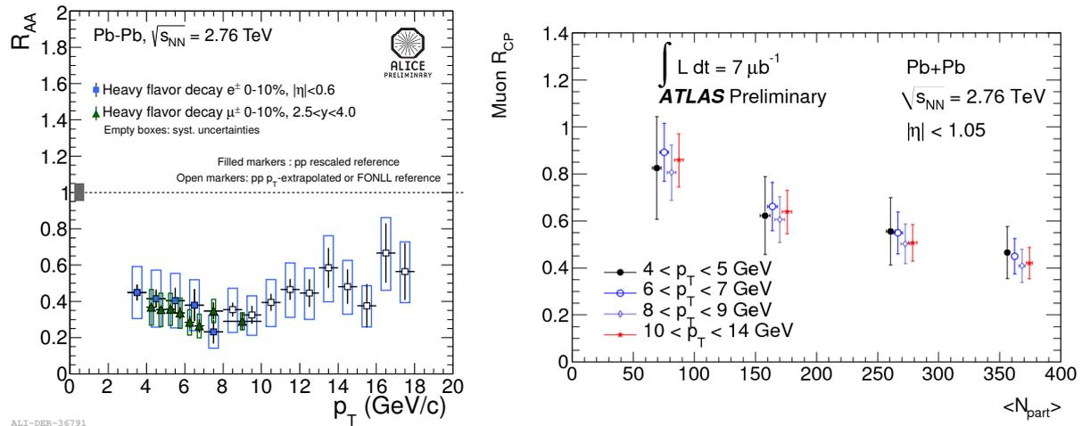
**Figure 3.** Suppression of heavy-flavour decay leptons at the LHC. Left: ALICE measurements of  $R_{AA}$  of heavy-flavour decay muons at forward rapidity [21] and electrons at central rapidity [23] in central (0–10%) Pb–Pb collisions, as a function of  $p_T$ . Right: ATLAS measurement of  $R_{CP}$  of heavy-flavour decay muons at central rapidity, as a function collision centrality [22].
