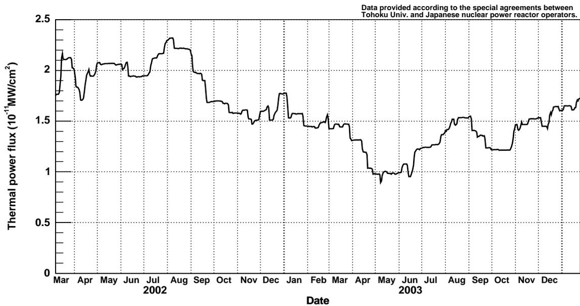
Figure 7.21: The thermal power flux from reactors at KamLAND.
