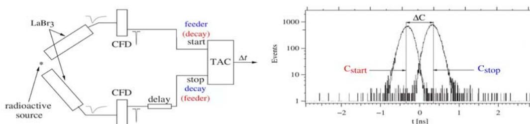
**Figure 4.** A simpler case of this experimental setup of just two detectors and the two time-distribution spectra are presented. Two time spectra can be produced depending on whether the decay gamma is providing the start (with the corresponding centroid,  $C_{\text{start}}$ ) or stop (with the corresponding centroid,  $C_{\text{stop}}$ ) signal (whether the feeder-gamma is providing the stop or start signal respectively).
