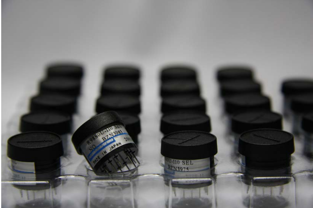
Figure 4.8: A picture of the HET Hamamatsu R9880U-110 SEL photomultipliers.
