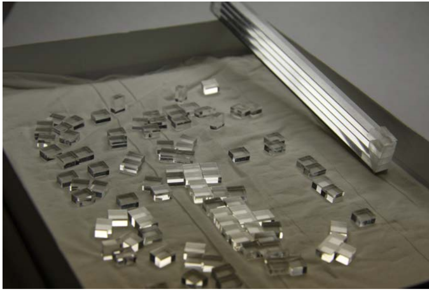
Figure 4.2: A picture of the HET plastic scintillators. At the top right there is a set of long scintillators.
