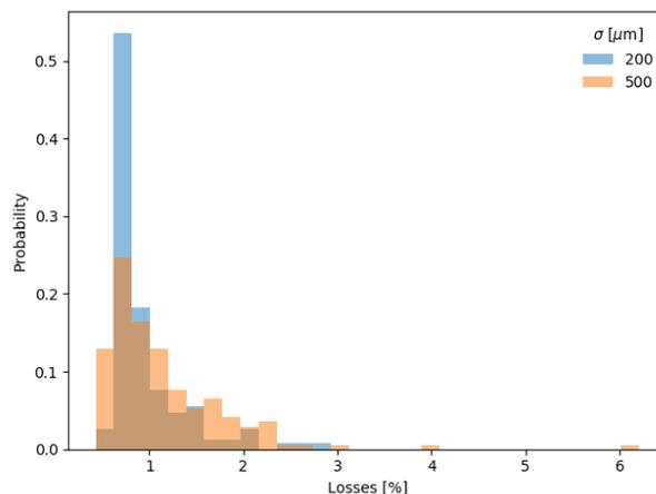
Figure 3: Distribution of losses after one iteration of the alignment procedure with 500 randomly sampled initial misalignment error seeds. Higher initial misalignments translate into more beam loss and greater variance.
