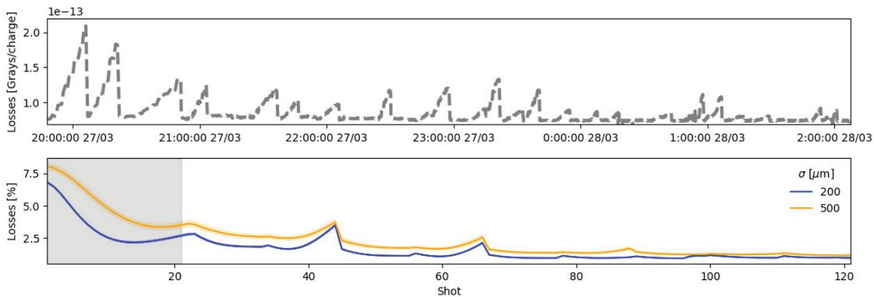
Figure 2: Top: Normalised BLM losses measured during the last alignment procedure over 6 hours for a single iteration of alignment during 2018 re-commissioning. Overall improvement was 31%. Bottom: 500 anode scan simulations with normally distributed initial misalignments. Average and 95% CI losses shown. Shaded area indicates girder scan with subsequent scans following ES tank anodes 1 to 5.
