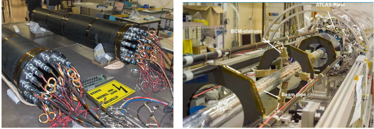
(a) The LUCID tubes before their installation. (b) The BCM in front of the ATLAS pixel detector around the beam pipe.
