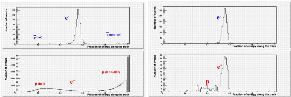
**Figure 1:** (*left*) Plot of the energy fraction released along the track in the calorimeter for both negative (top) and positive (bottom) charge in the rigidity interval  $20 \div 30$  GV. (*right*) The same distributions after applying an energy-momentum match condition and topological cuts related to the shower profile.
