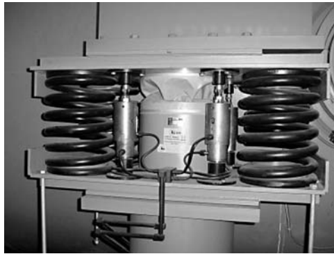
Fig. B11.2. View of an elastic unit with springs, damper and mechanical fuses
