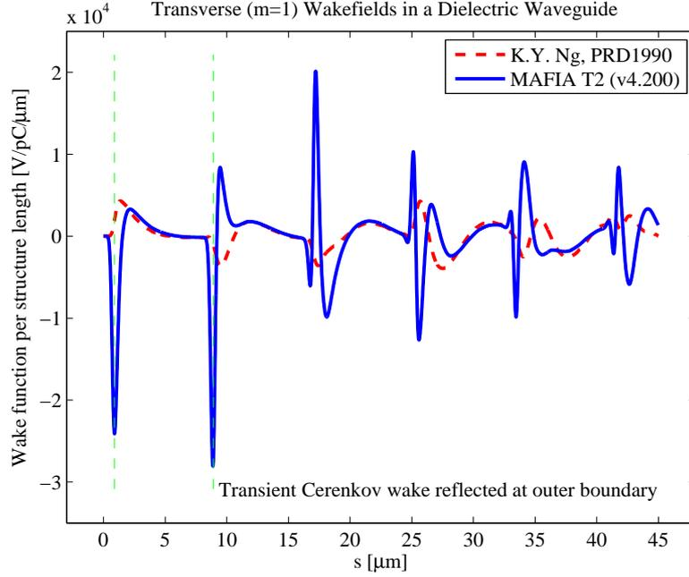
**FIGURE 1.** Wake functions for a dielectric waveguide, normalized to structure length, as a function of the distance behind the bunch-head: MAFIA vs. analytical calculation. The vertical dashed lines indicate the expected separation between the initial transient pulse and its reflection at the outer conducting boundary.
