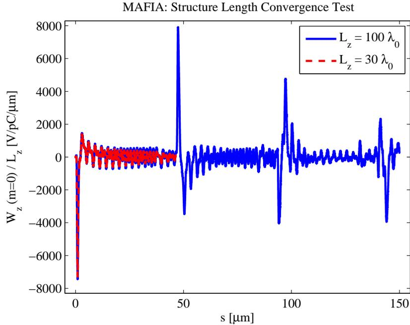
**FIGURE 3.** Longitudinal (monopole) wakefields in a Bragg fiber obtained using MAFIA for two structure lengths:  $30\lambda_0$  and  $100\lambda_0$ . The reflected transient pulse appears to decrease with distance behind the bunch.
