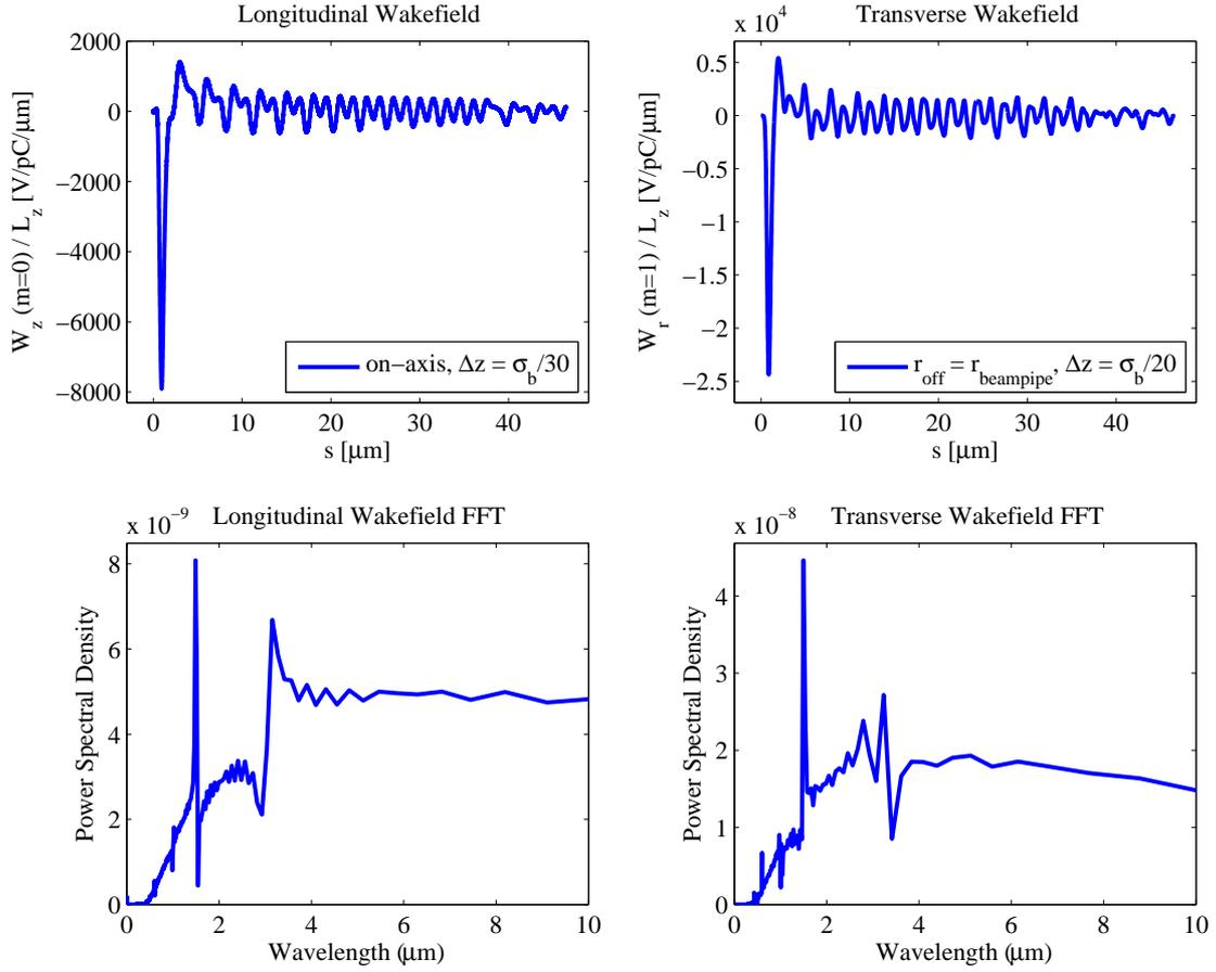
**FIGURE 2.** Wake functions in a Bragg fiber obtained using MAFIA. The top row shows the longitudinal (monopole) and transverse (dipole) wake functions, normalized to structure length ( $L_z = 30\lambda_0$ ), while the bottom rows show the corresponding Fourier transforms.
