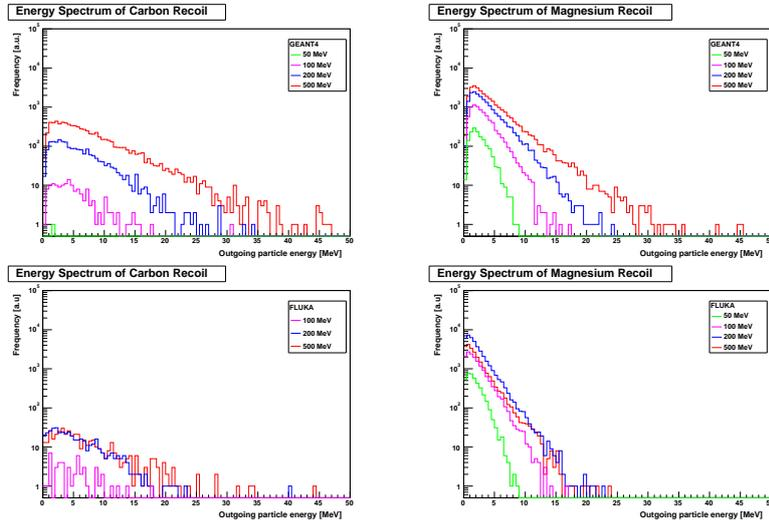
Fig. 2 – Energy spectrums of carbon and magnesium recoils for 50, 100, 200 and 500 MeV protons on silicon. GEANT4 simulation (top) and FLUKA simulation (bottom).
