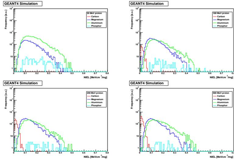
Fig. 5 – NIEL spectra for carbon, magnesium, aluminium and phosphorus recoils produced by 50, 100, 200 and 500 MeV protons on silicon by using GEANT4 tool.
