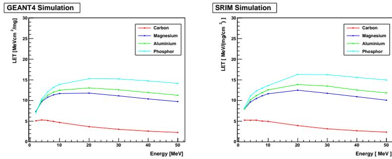
Fig. 3 – LET spectrums of some recoil heavy ions produced by 50, 100, 200 and 500 MeV protons on silicon. GEANT4 simulation (left) and SRIM simulation (right)
