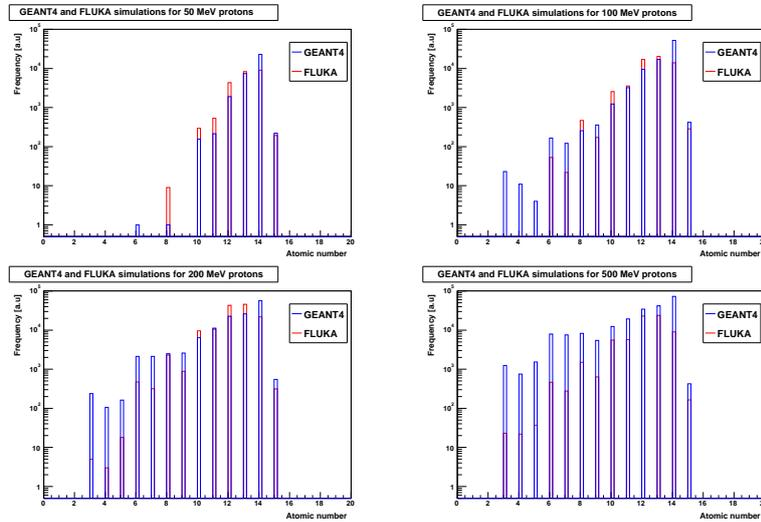
Fig. 1 – Recoil spectrums as a function of atomic number for 50, 100, 200 and 500 MeV protons on silicon by using GEANT4 and FLUKA tools.
