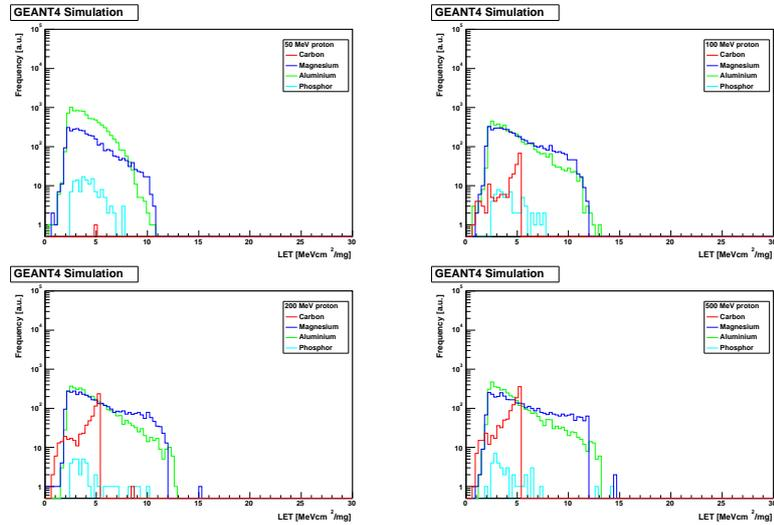
Fig. 4 – LET spectrums for carbon, magnesium, aluminium and phosphorus recoils produced by 50, 100, 200 and 500 MeV protons on silicon by using GEANT4 tool.
