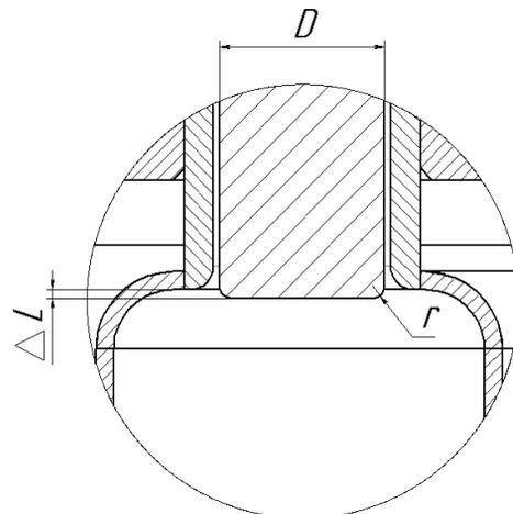
Figure 4: The most important parameters of FTS plungers.
