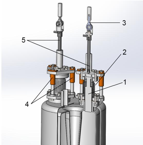
Figure 2: Concept of the Frequency tuning system based on mobile plungers in the end caps holes of HWR.
