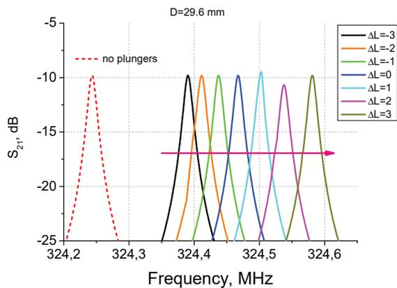
Figure 5: The simulated frequency dependencies of  $S_{21}$  of HWR without plungers (dashed line) and with plungers of diameter  $D = 29.6$  mm and various penetration depth  $\Delta L$  (solid lines).
