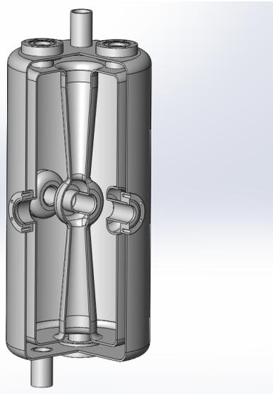
Figure 1: 324 MHz HWR cavity model.
