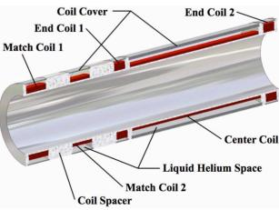
Figure 3: Spectrometer solenoid cold mass assembly.
