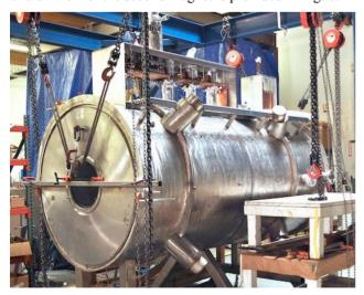
Figure 6: Second spectrometer solenoid nearly completed.
