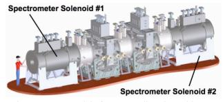
Figure 1: CAD model of MICE cooling channel layout.
