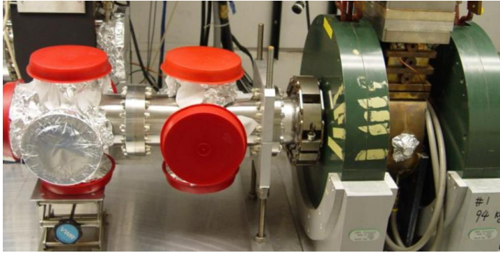
FIGURE 1. \frac{1}{2} cell, 1.3 GHz electron injector with a diagnostics chamber.
