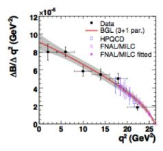
**Figure 4:** Combined fit to BABAR data and LQCD points to extract  $|V_{ub}|$ .
