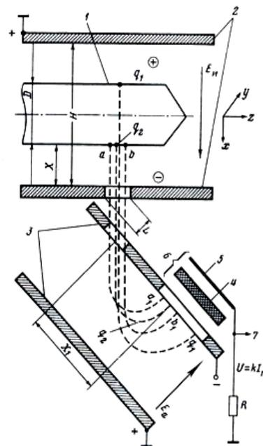
Figure 2: BCSM scheme, 1-Particle beam, 2-Ion extractor with slit, 3-Electrostatic analyzer, 4-MCP image
