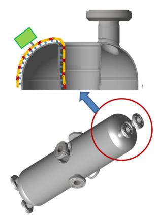
Figure 11: The flexible T-map system fits on a 162.5 MHz  $\beta$  = 0.12 half-wave-resonator.
