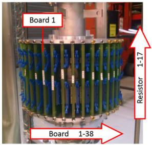
Figure 3: Photograph of the Cornell single-cell T-Map system which works for 1.3 GHz ILC-shape and Cornell ERL-shape cavities.
