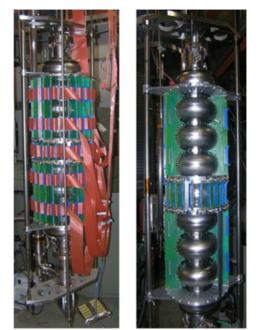
Figure 4: Photograph of the Cornell multi-cell T-Map system.
