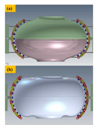
Figure 9: The flexible T-map system fits on (a) a 1.3 GHz ILC-shape SRF cavity; (b) a 1.3 GHz re-entrant shape SRF cavity.
