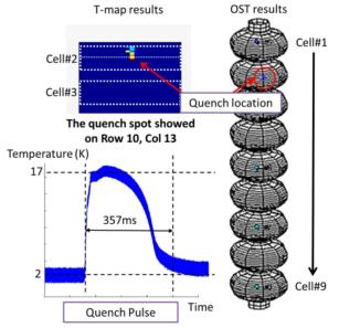
Figure 6: Quench location with TB9AES022 detected by the OST system and the Cornell T-Map with the quench recorded by the T-Map system shown in the inset on the left.
