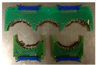
Figure 2: A 3-cell board and a 1-cell board from the Cornell T-Map systems.
