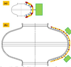
Figure 10: The flexible T-map system fits on (a) a 3.9 GHz elliptical SRF cavity; (b) a 650 MHz elliptical SRF cavity.
