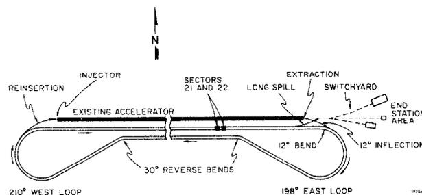
FIG. 1--Schematic layout of recirculation system.
