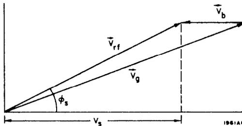
FIG. 6--Vector diagram showing the addition of the generator voltage  $V_g$  and the beam induced voltage  $V_b$  to result in the final RF voltage  $V_{RF}$  where  $\phi_s$  is measured from the wave crest.
