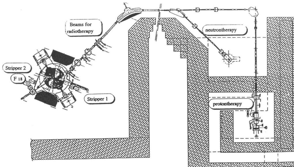
Fig 1 : MEDICYC 65 MEV H<sup>-</sup> cyclotron for neutrontherapy, low energy protontherapy and F<sup>18</sup> production.
