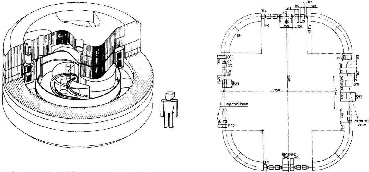
Fig 5 : Cut away view of the superconducting cyclotron and general layout of the SFM synchrotron proposed for EULIMA.
