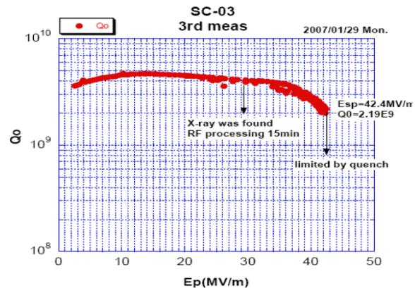
Figure 5: Measured  $Q_0$  of the 1.3 GHz single cell.
