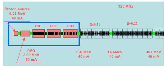
Figure 7: Sketch of the 325 MHz linac for CIADS.
