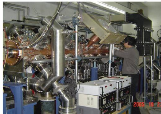
Figure 2: The 3.5MeV RFQ accelerator.
