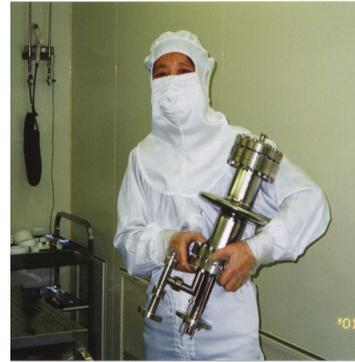
Figure 4: 1.3 GHz single cell at  $\beta=0.45$ .
