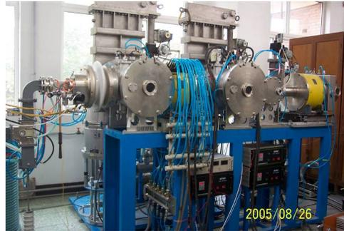
Figure 1: High intensity ECR ion source.
