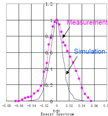
Figure 3: The Beam energy spectrum of the RFQ.
