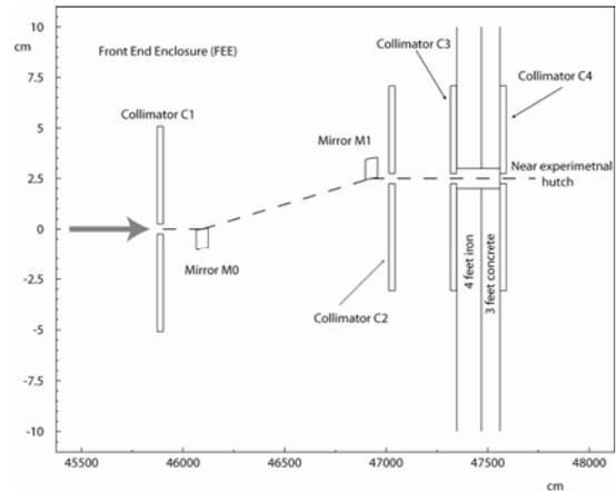
Fig.1: Schematic view of the mirror system
