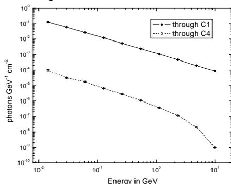
Fig. 3: Energy spectra of photons passing through C1 and C4 respectively. Collimator C2 out
