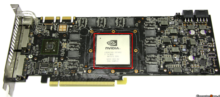
Figure 3.1: This picture shows a typical graphics card with its GPU in the middle [10].
