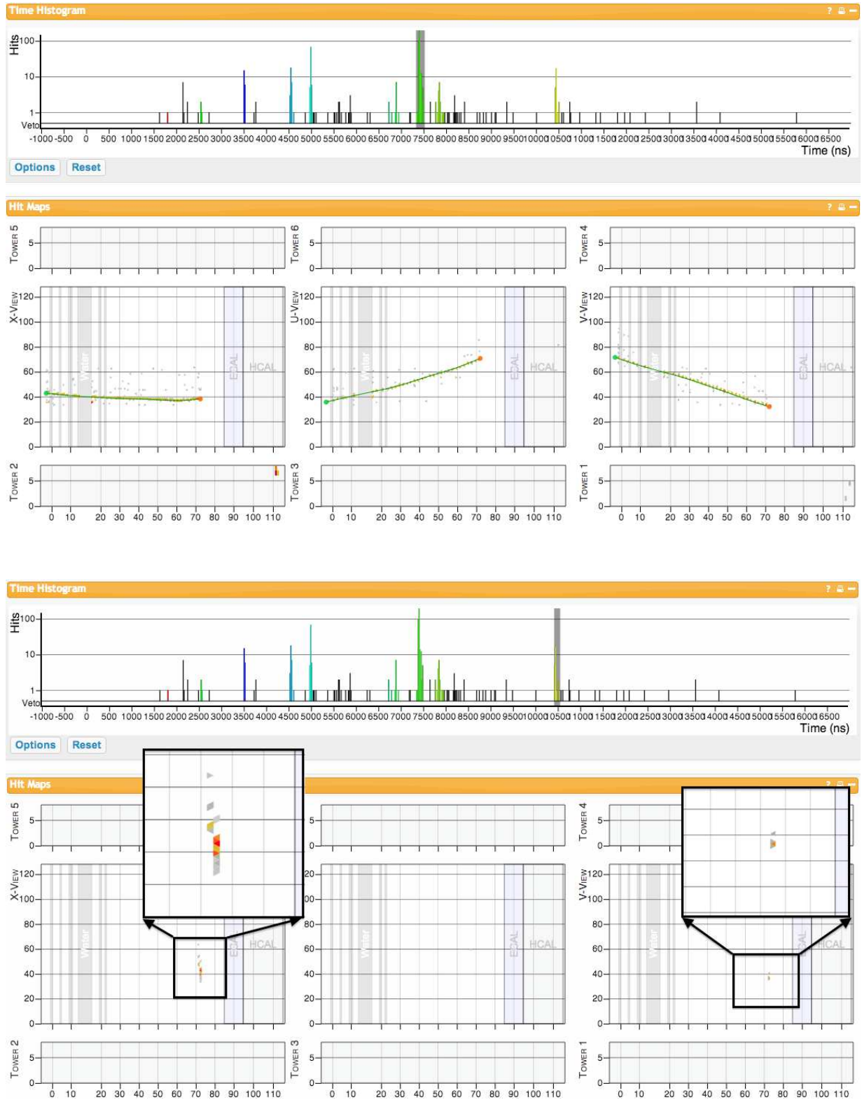
FIG. 5.15: An example of a TwoView Michel electron in Run 2000, Subrun 1, Gate 583. The upper plot shows a muon track stopping in fiducial in timeslice 8. The lower plot shows the TwoView Michel electron in X and V view in timeslice 10.
