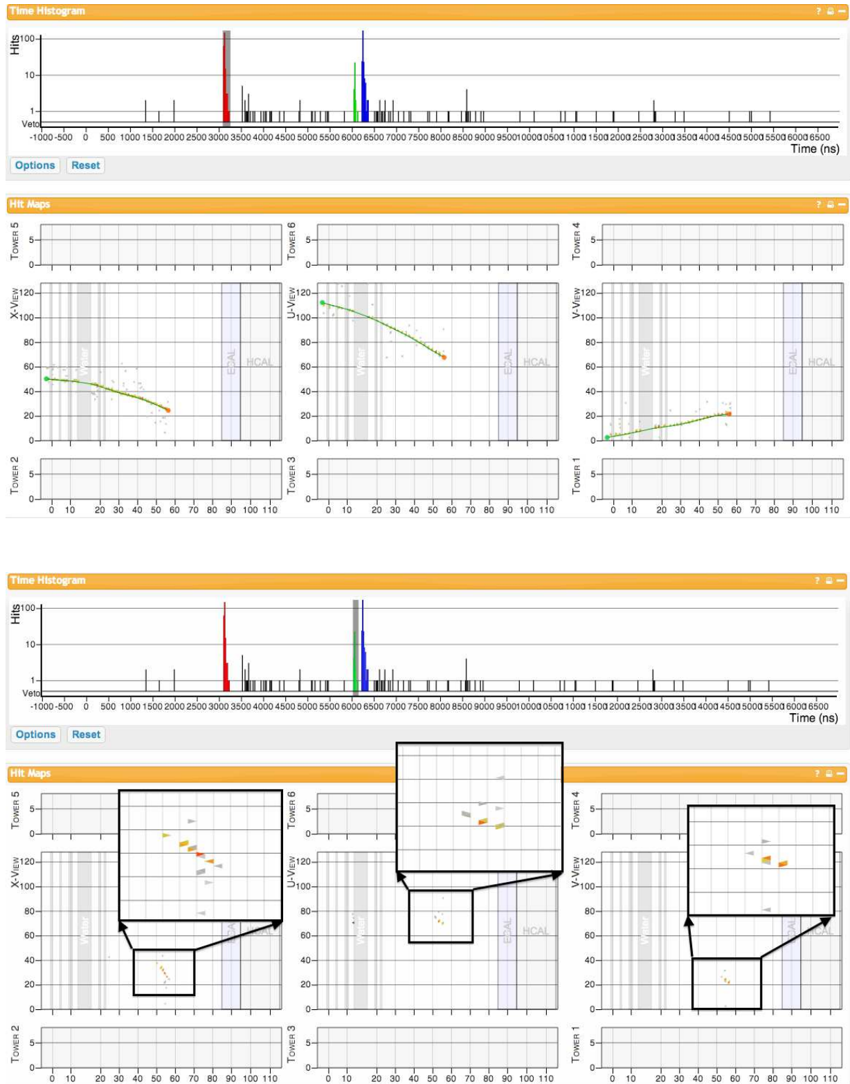
FIG. 5.16: An example of a ThreeView Michel electron in Run 2000, Subrun 1, Gate 80. The upper plot shows a muon track stopping in fiducial in timeslice 1. The lower plot shows the ThreeView Michel electron found in all three views in timeslice 2.
