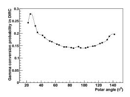
FIG. 1: Gamma conversion probability in DIRC as a fuction of polar angle  $(\theta)$  for 1 GeV photons
