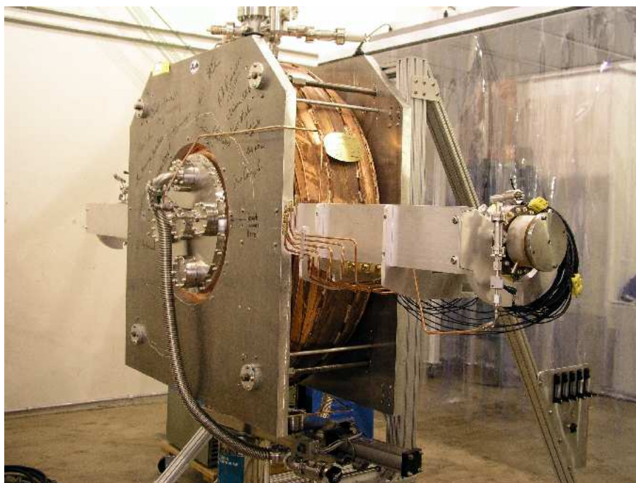
Figure 43: (Color) 201 MHz rf cavity. The 1.4-m-diameter cavity has curved Be windows and is provided with a thin exit port to permit dark current studies.
