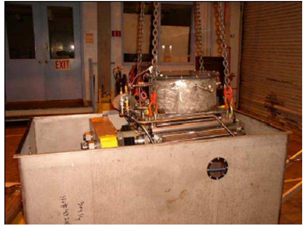
Figure 41: (Color) (Left) 15-T MERIT solenoid under test at MIT. Three nested coils permit operation at 5, 10, and 15 T. The coils are normal conducting but cooled to liquid-nitrogen temperature to ease the requirements on the power supply. (Right) Hg-jet syringe pump system being placed in containment vessel at ORNL.
