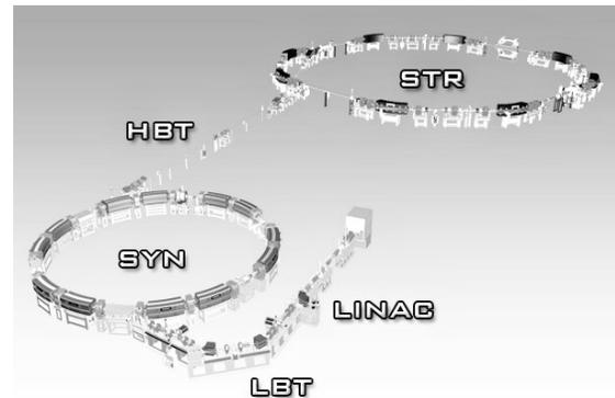
Figure 1: SPS accelerator complex.
