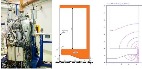
Figure 2: Present RF cavity of the storage ring.
