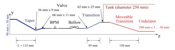
Figure 1: Schematic presentation of the tapered transition in front of the in-vacuum undulator.
