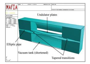
Figure 2: Model of the IVU tank with two movable transitions for the MAFIA calculations. In the model the vacuum tank is assumed to be only 0.4 m long. The tapers have the correct lengths. An undulator gap of 6 mm is considered.
