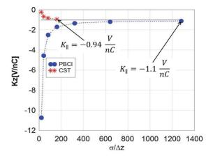
Figure 6: Numerical error and convergence rate of CST PS for different mesh resolutions in the 6mm gap case.
