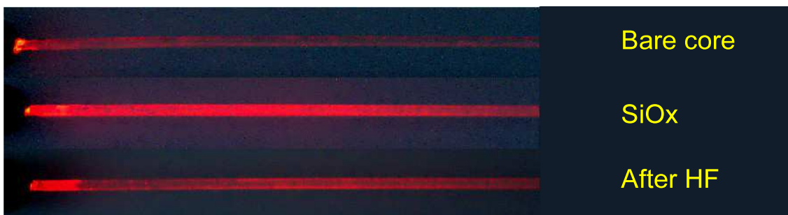
Figure 4. Example of dark field pictures of a fiber coated with a thin \text{SiO}_x film (200 nm). Top image: uncoated fiber, middle image: fiber after coating, bottom image: coated fiber after exposure to HF vapors.
