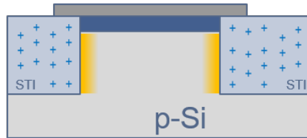
Figure 2. Cross section of a transistor along the line indicated in figure 1. The channel of the parasitic transistor along the STI is indicated in yellow.
