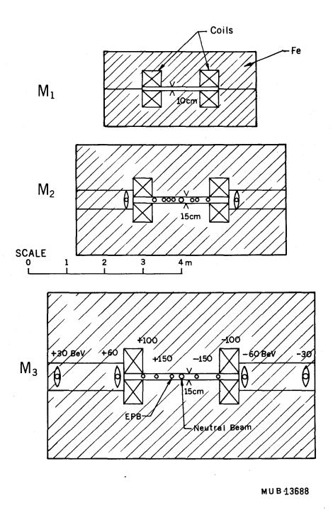
Fig. 2. Cross sections of targeting magnets  $\mathbf{M}_1\text{, }\mathbf{M}_2\text{, and }\mathbf{M}_3\text{.}$
