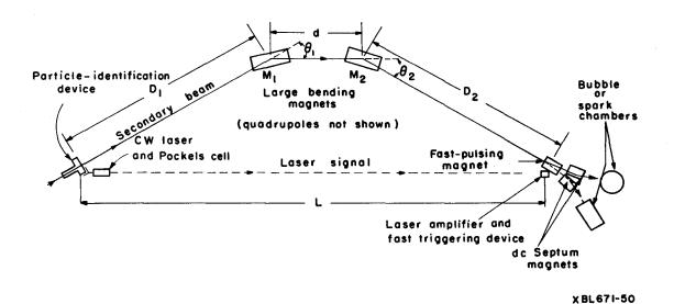
Fig. 1. Illustration of technique for separating particles with fast-pulsing magnets.
