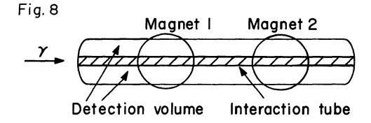
Fig. 8. Possible streamer chamber arrangement. Counters are triggered according to specific reaction.
