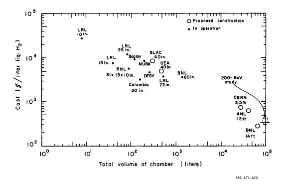
Fig. 2. Cost per unit volume of cryogenic bubble chambers as a function of the total volume.
