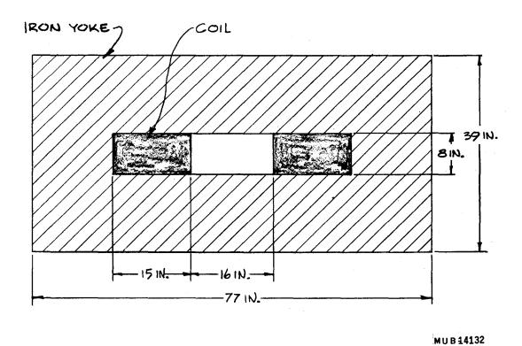
Fig. 1. Conventional picture-frame magnet, capable of about 20,000 G.
