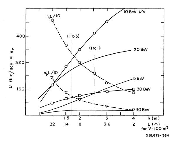
Fig. 1. Neutrino interactions per day in liquid  $H_2$  vs the radius of a cylindrically shaped  $H_2$  chamber. The solid lines show the interactions per day per meter for a given radius and the dotted lines show the interactions per day for a fixed volume of 100 m<sup>3</sup>.  $\pi \rightarrow \nu$  in a 1000-m beam. The ordinate is interactions per meter per day.
