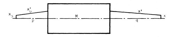
Fig. 1. Illustration of the relevant quantities arising in the transport of a particle through the magnet system M.
