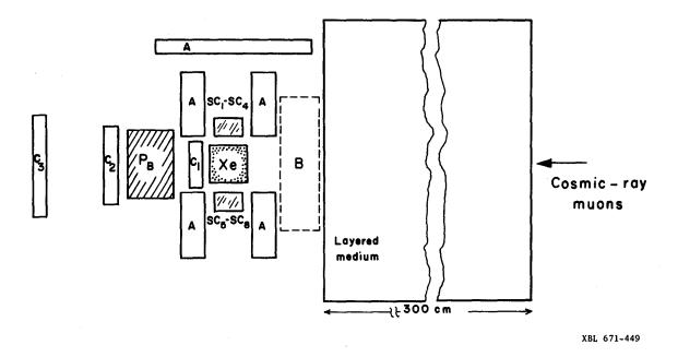
Fig. 4. Alikhanyan's apparatus for the detection of resonance radiation. For explanation of symbols, see text.
