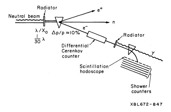
Fig. 9. Tagged photon beam with two conversion stages used.
