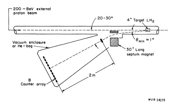
Fig. 3. A possible experimental configuration for measuring particle production at 180 deg in the laboratory system.
