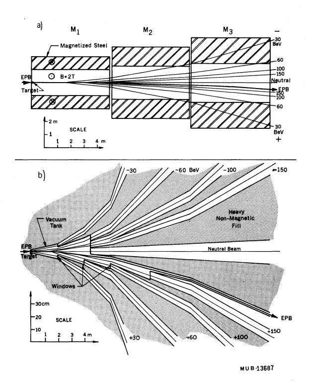
Fig. 1. (a) Plan view of EPB targeting magnets.
