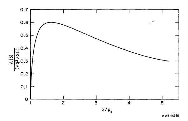
Fig. 4. Momentum-dependent part of channel-transmission function.
