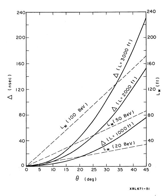
Fig. 2. Difference in transit time,  $\Delta$ , between arrival of the particle and trigger signal vs total bending angle ( $\theta$ ). Values for total magnet lengths ( $M_1$  plus  $M_2$ ) in feet are the same as the transit-time difference values.
