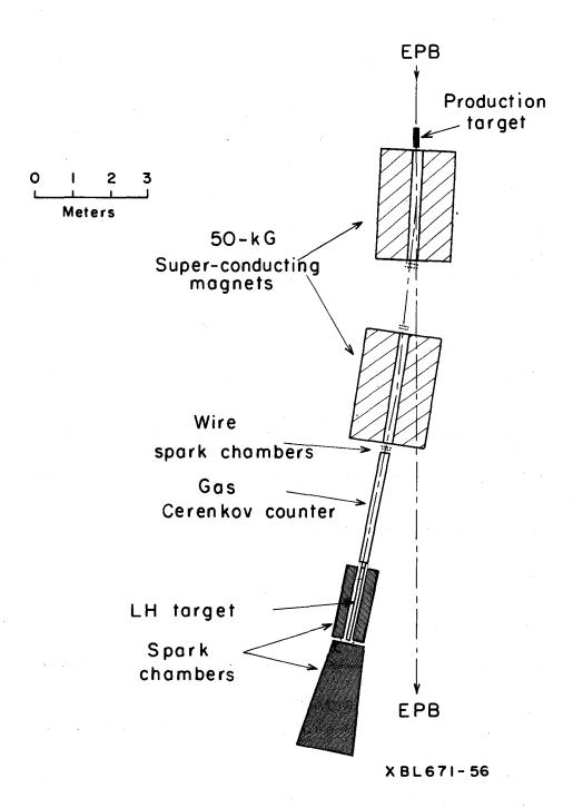
Fig. 4. Schematic layout for 50-BeV/c secondary beam. Bend is 5 deg in each magnet.
