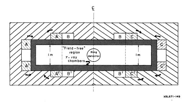
Fig. 3. Elevation of section A-A', Fig. 2, showing coils A-A', C-C', and bucking coils B-B' used to obtain a field-free region. Yoke may not be needed over field-free region.
