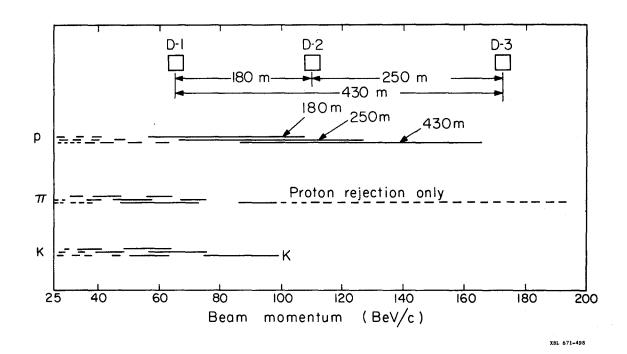
Fig. 1. Momentum pass bands (indicated by the extent of the horizontal lines) for best-two-out-of-three deflector system with circular polarization (cancellation of deflection for wanted particle). Here f = 10 GHz. The pass band corresponds to the region for which the deflection of the least-deflected contaminant is greater than or equal to the deflection imparted by a single deflector. Deflector spacings of 180 and 250 m are shown.
