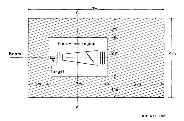
Fig. 2. Schematic diagram illustrating the proposed way of using the Cerenkov ring detector in combination with a magnetic field. Shading indicates magnetic field.
