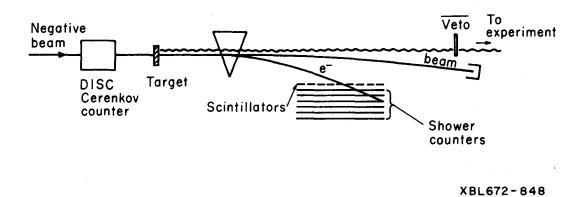
Fig. 10. Detail of tagged  $\gamma$ -ray experiment.
