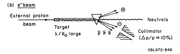
Fig. 8. Schematic representation of realization of (a) photon beam and (b) electron beam.
