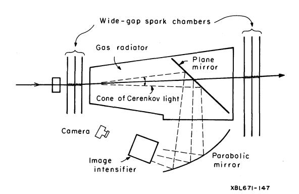
Fig. 1. Cerenkov ring-image detector, with trajectory-defining spark chambers before and after.
