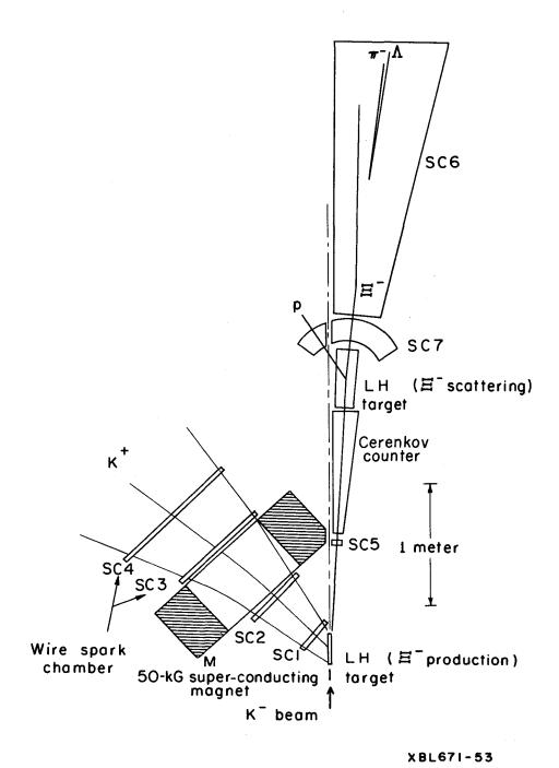
Fig. 1. Possible experimental setup for production and scattering of  $\Xi^-$ .
