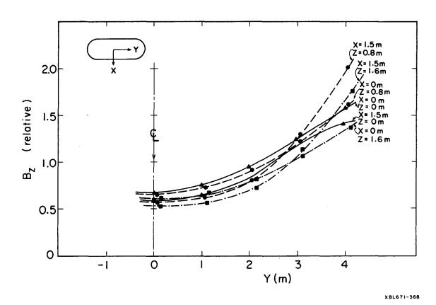
Fig. 8. B<sub>z</sub> vs Y for X = 0 and 1.5 m and for Z = 0.0, 0.8, and 1.6 m for the race-track configuration proposed for the magnet for the 100 m<sup>3</sup> hydrogen chamber. B<sub>z</sub> (kG) is ordinate x (NI) x 10-6.
