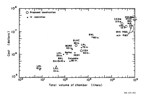
Fig. 1. Total costs of cryogenic bubble chambers as a function of the total volume.
