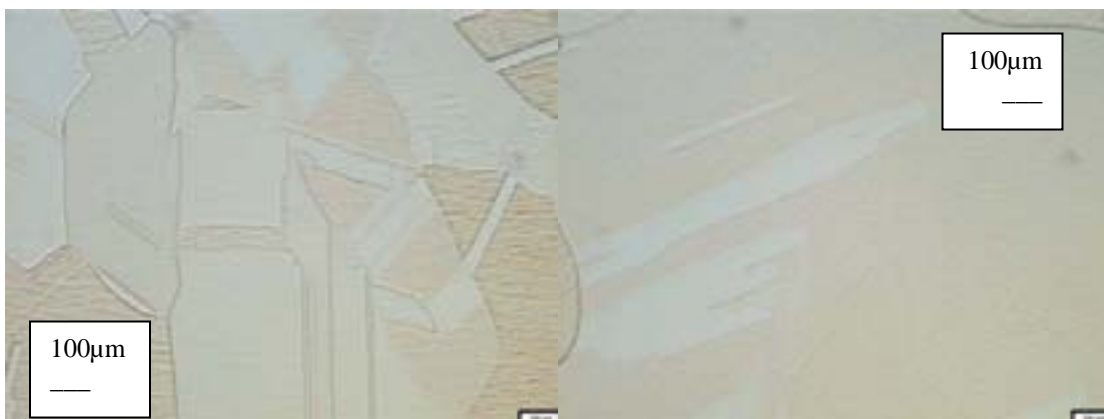
Figure 8: Grain structure of samples at 25x magnification. Control (left) has an overall smaller grain size than the experimental sample (right).
