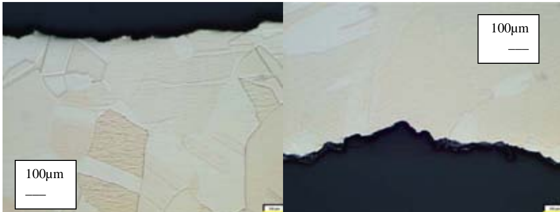
Figure 6: Inner edge of absorber at 25x magnification showing water corrosion. The experimental (right) shows greater damage.
