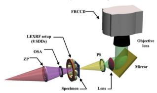
Figure 1: STXM mode as implemented on TwinMic.
