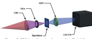
Figure 2: TXM mode as implemented on TwinMic.
