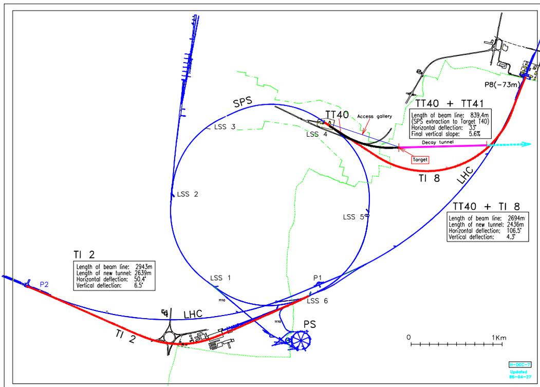
**Figure 1 :** Overview of the SPS complex with the new transfers lines TT40, TT41, TI8 (extraction from LSS4) and TI2 (extraction from LSS6) [LSS = Long Straight Section].
