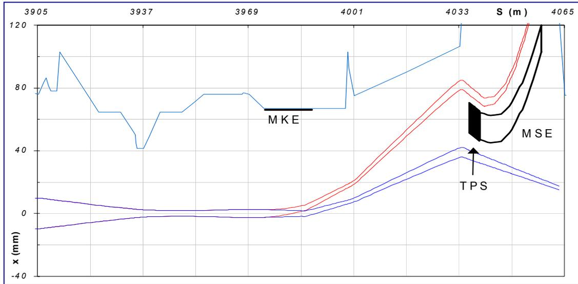
**Figure 4:** Extraction channel layout for the horizontal plane in LSS4. The circulating beam (blue) is bumped horizontally close to the septum using 4 horizontal bumper magnets and kicked into the extraction channel by the MKE kicker magnet (red trace).
