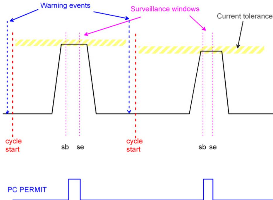
**Figure 10** : Power converter surveillance windows and PERMIT signal. sb and se refer to the limits of the surveillance window.
