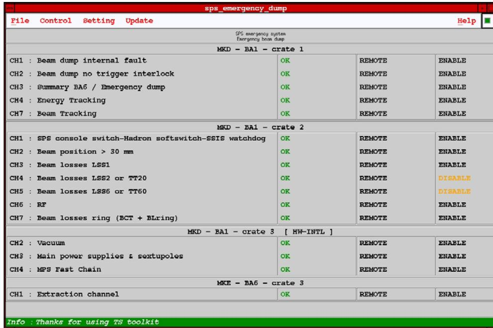
**Figure 2 :** User interface of the SPS Emergency Interlock System in the control room with the list of presently available interlock channels. The “remote” flag indicates that a channel can be disabled by the operator. In this example channels 4 and 5 have been disabled by the operator.
