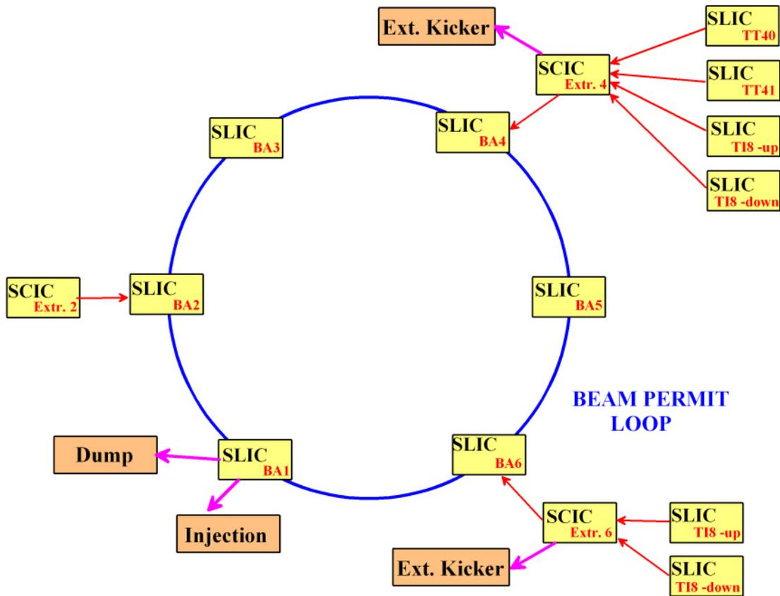
**Figure 9** : Architecture of the SPS hardware interlock system, including the beam and extraction interlock systems.
