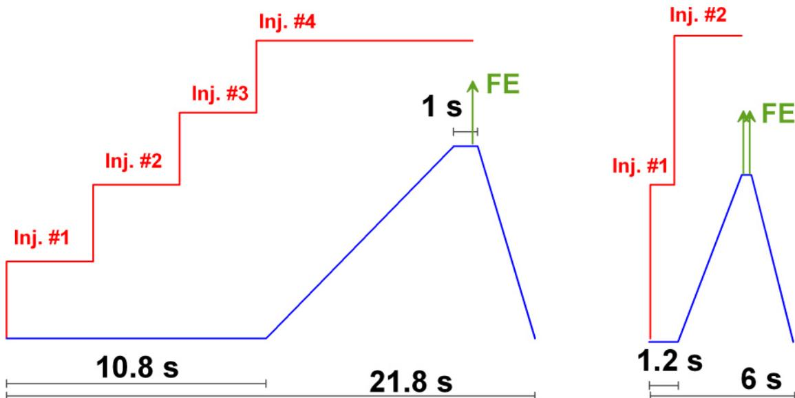
**Figure 3** : Examples for LHC (left) and CNGS (right) beam cycles in the SPS. The blue line represents the beam momentum (respectively the magnetic field), while red lines indicate the total beam intensity.
