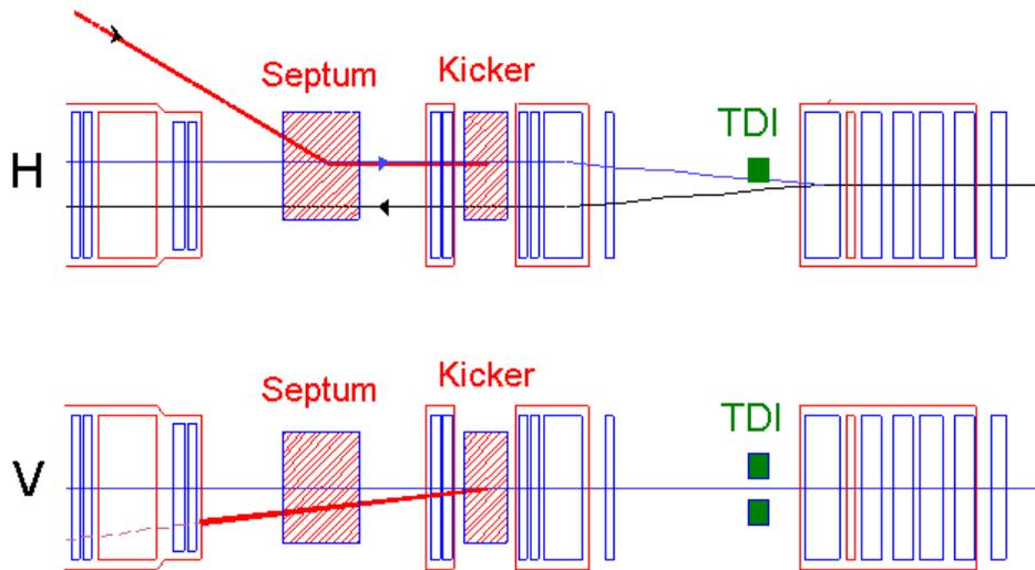
**Figure 12 :** Layout of the LHC injection area. The septum magnet deflects the beam horizontally while the kicker provides a vertical kick. If one or more kicker modules mis-fire, the beam hits the TDI absorber block.
