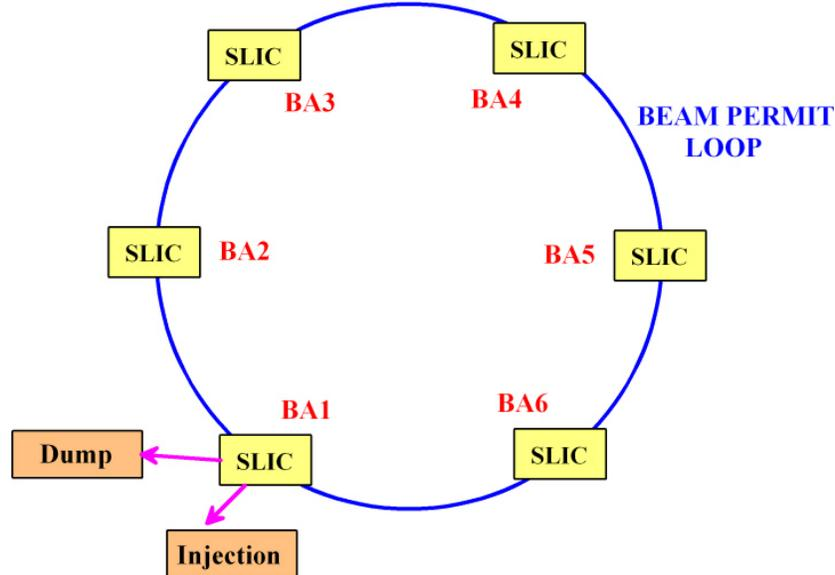
**Figure 6 :** Architecture of the SPS beam interlock system. One SLIC module must be installed in each SPS access point. All SLIC modules are connected to the BEAM PERMIT LOOP. The state of the BEAM PERMIT LOOP is forwarded to the SPS beam dump and injection kickers.
