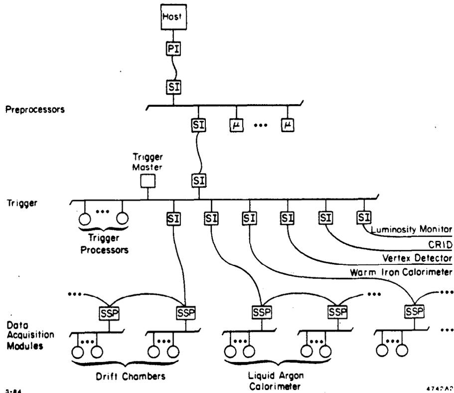
Figure 4. SLD Data Acquisition System
