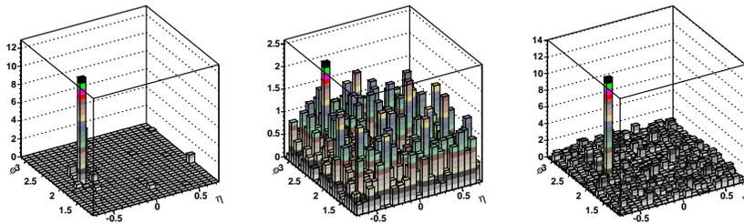
Figure 2: Energy distribution vs.  $\eta$  and  $\phi$  in EMCal acceptance. One cell corresponds to  $5 \times 5$  EMCal towers ( $\Delta\eta \times \Delta\phi \sim 0.070 \times 0.070$ ). Left: 55 GeV PYTHIA generated jet; center: HIJING event with  $b \sim 5$  fm.; right: superposition of the two events. Note variation of vertical scale.
