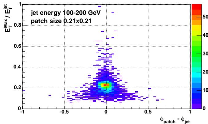
Figure 3: Comparison of L1 trigger algorithm and PYTHIA internal jet finder for PYTHIA events containing  $100 < E_T < 120$  jets and L1 patch size  $0.21 \times 0.21$ . Plot shows ratio of  $E_T$  vs. difference in angle for the two algorithms.
