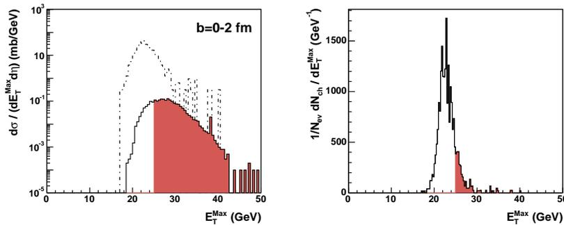
Figure 7: PYTHIA+HIJING,  $b=0-2$  fm (central collisions), jet patch  $0.21 \times 0.21$ . Left:  $E_T^{\text{Max}}$  differential cross section for background (dash-dot) and for background plus 50-60 GeV jets (solid). Filled area shows 80% of embedded jet yield. Right:  $E_T^{\text{Max}}$  distribution for the background events weighted by charged multiplicity in TPC, which is proportional to data volume. Filled area shows fraction of data volume that contains 80% of jet yield.
