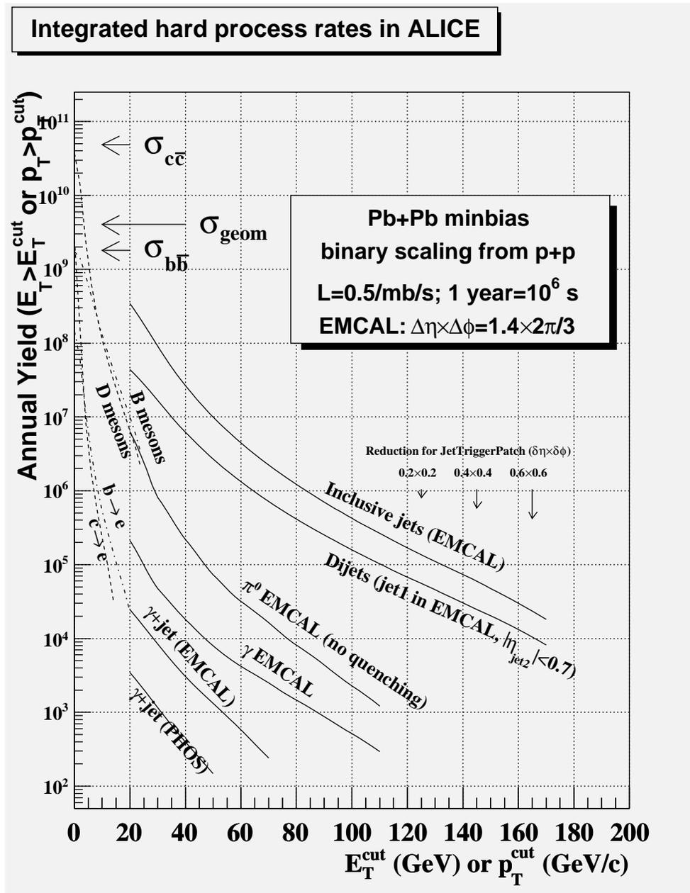
Figure 1: Hard process annual yields ( $10^6$  seconds) in ALICE acceptance for minbias Pb+Pb at nominal luminosity. Calculations derived from [3, 4, 5, 6]. Vertical arrows indicate yield reduction due to EMCAL acceptance for various jet trigger patch sizes.
