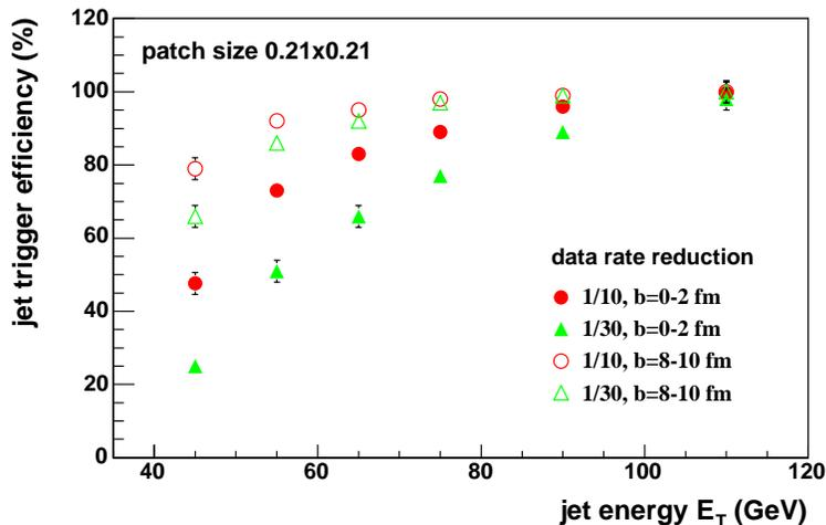
Figure 10: PYTHIA+HIJING: jet trigger efficiency as a function of jet energy for central and peripheral collisions, for a  $0.21 \times 0.21$  patch with data rate reduction of 1/10 and 1/30.
