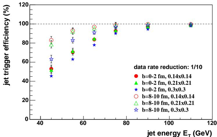
Figure 12: PYTHIA+HIJING: jet trigger efficiency vs. energy for 1/10 reduction in data rate, for various patch sizes and central and peripheral collisions.
