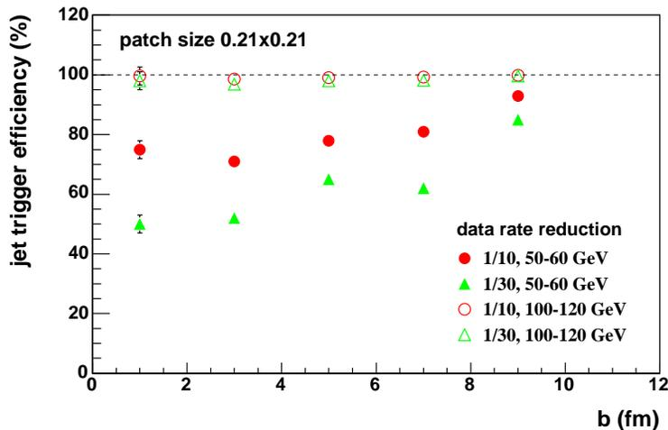
Figure 11: PYTHIA+HIJING: jet trigger efficiency as a function of impact parameter for two jet energies, for a  $0.21 \times 0.21$  patch with data rate reduction of 1/10 and 1/30.
