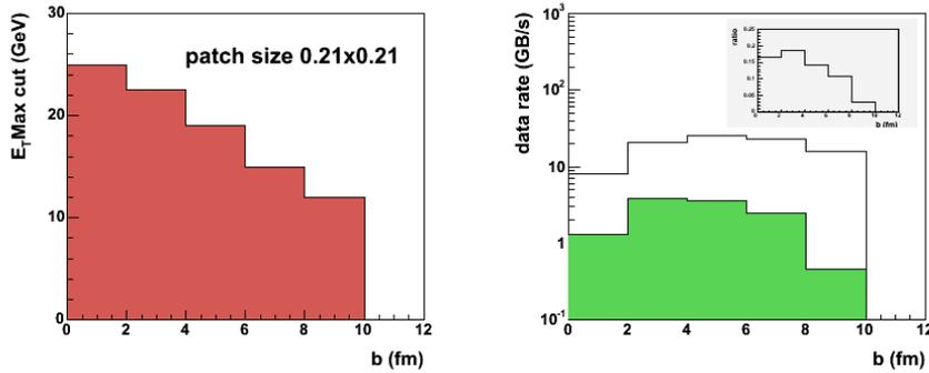
Figure 9: PYTHIA+HIJING, jet patch  $0.21 \times 0.21$ , jet  $E_T=50-60$  GeV. Left: impact parameter dependence of  $E_T^{\text{Max}}$  cut required for 80% jet efficiency. Right: impact parameter dependence of L1 input (upper histogram) and output (lower filled histogram) data rate using cuts in left panel. Insert shows their ratio.
