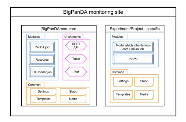
Figure 1. Module structure of BigPanDA monitoring package for an experiment/project.
