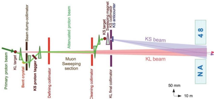
Fig. 5.13. Schematic layout of the  $K^0$  beams.
