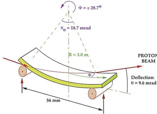
Fig. 5.14. Schematic arrangement of the bent crystal [31].
