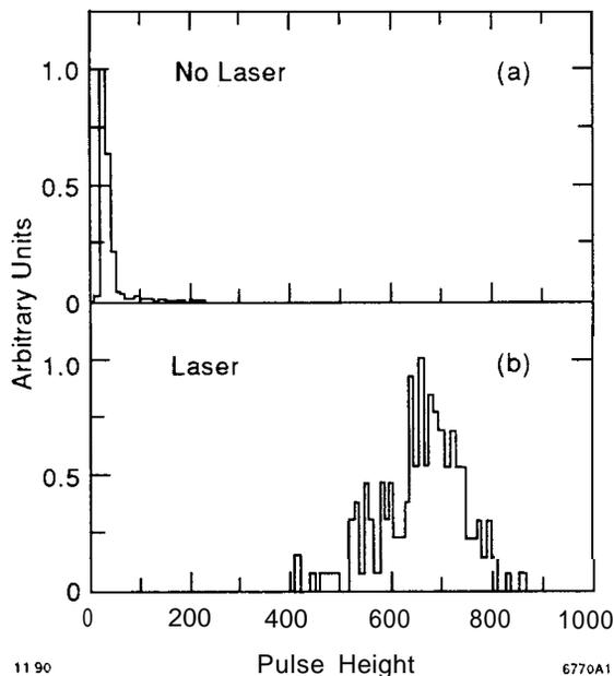
**Figure 10:** Pulse height distribution from the Cerenkov detector in the Compton Polarimeter: (a) no laser light; (b) 1aser light colliding with electron beam.
