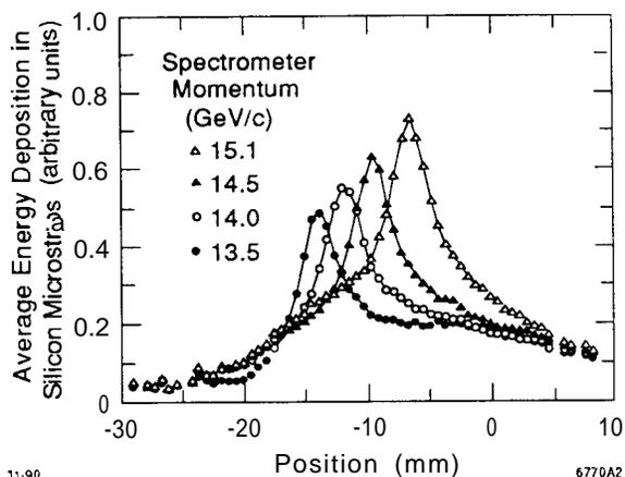
**Figure 8:** These data were taken with four different settings of the spectrometer central momentum (13.5 → 15.1 GeV/c.) The detector acceptance was  $\Delta P/P \approx 8\%$ . The expected scattering angle momentum dependence for  $ee$  scattering predicts  $A_y \sim 4.3 \text{ mm} * A_P \text{ (GeV)}$  at the Møller detector.
