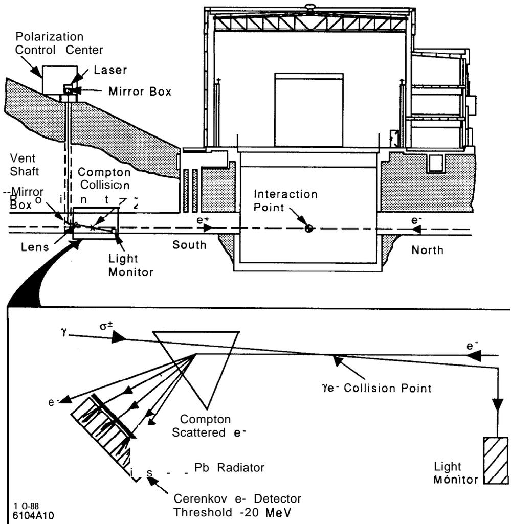
**Figure 9:** Location of the SLC Compton polarimeter components is shown. The light from the laser on the surface is directed into collision with the electron beam after it has passed through the interaction point.
