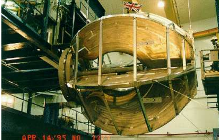
Figure 3.12: Photograph of the CLAS Superconducting Toroidal Magnet. Image source: [47].
