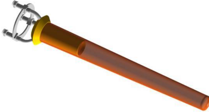
Figure 3.10: A schematic diagram of the g11a Cryotarget. The cryotarget cell used for the g11a run period was designed by Steve Christo [45]. It was 40 cm long, 4 cm in diameter and filled with liquid H_2 . Image source: [45].
