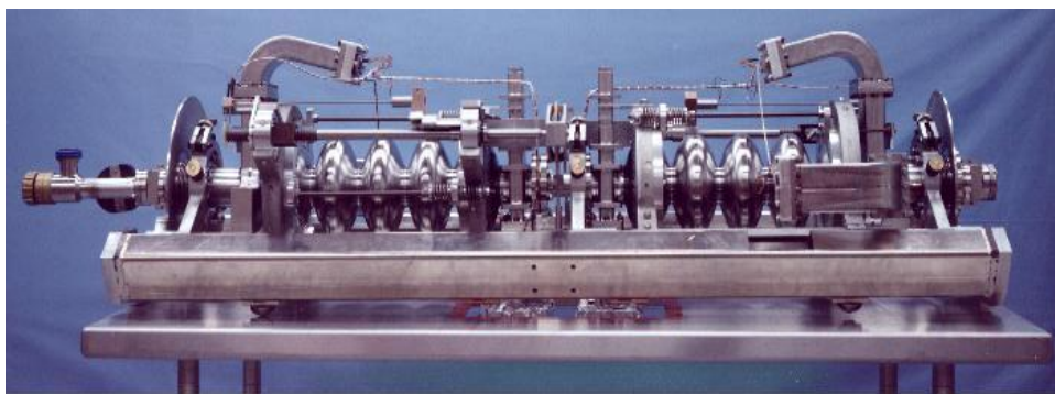
Figure 3.3: Shown above is a pair of superconducting niobium RF cavities. The cavities are the innermost component characterized by the elliptical bulges perpendicular to the beam line. Image source: [38].
