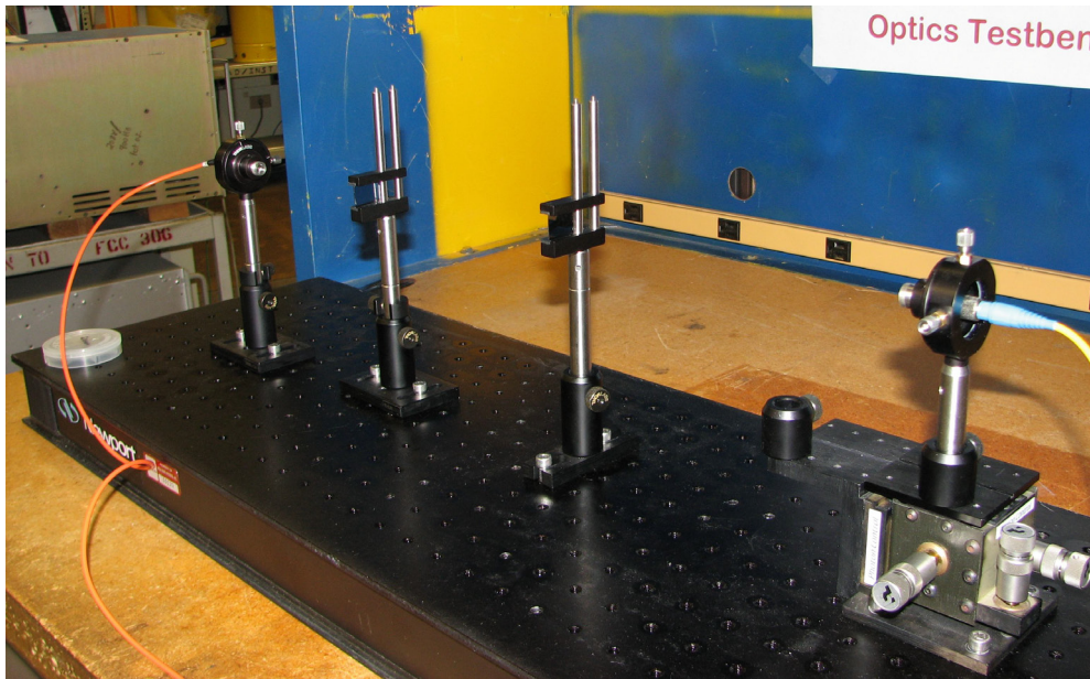
Figure 3: Free-space optical path implemented on an optical breadboard. On the right is the transmitter end with single mode fibre and launching lens. On the left is the receiver end with multimode fibre and receiving lens. In between are two swinging gates with doped silicon samples.
