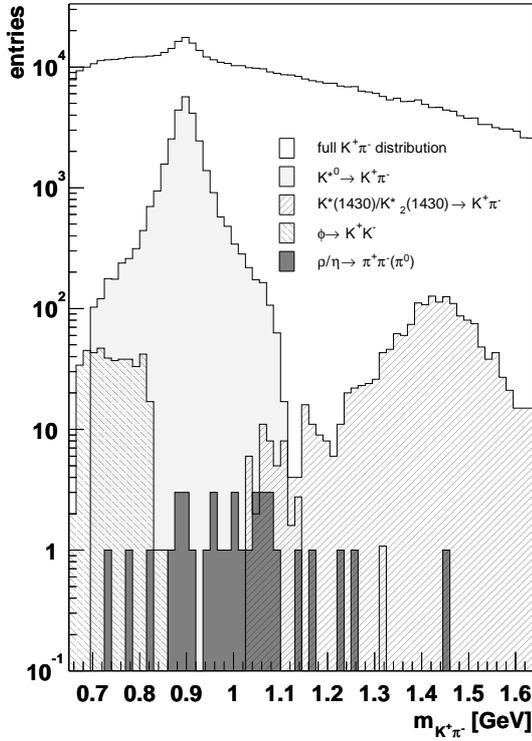
**Figure 4.16:** Expected contributions from resonances to the  $K^+\pi^-$  invariant mass distribution. To select the daughter tracks of the resonances, the Monte-Carlo track matching method is used.
