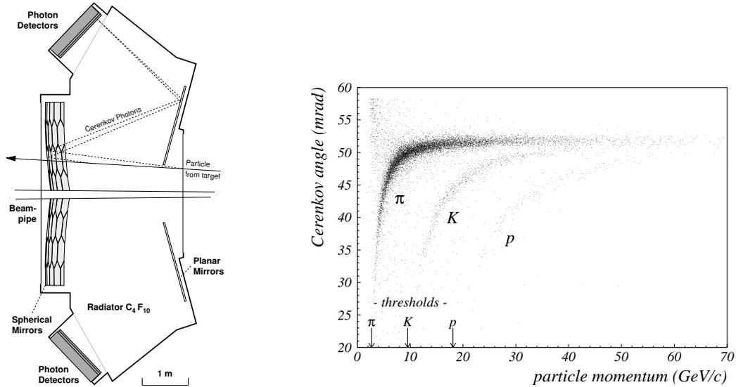
**Figure 3.9:** Left: Schematic side-view of the RICH detector. Right: Measurement of the Čerenkov angle as a function of momentum for different particles. The Čerenkov thresholds for pions, kaons, and protons are indicated by the arrows. Both from [ari04].
