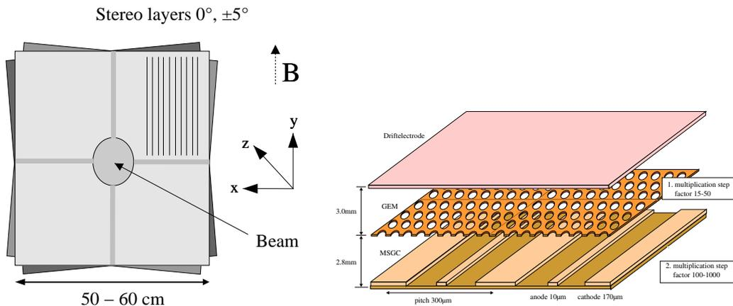
**Figure 3.7:** Front view of an ITR superlayer (left) and schematic view of an ITR chamber (right). The readout layer on the bottom is covered by the GEM foil. The drift cathode layer is shown on top [zie98].
