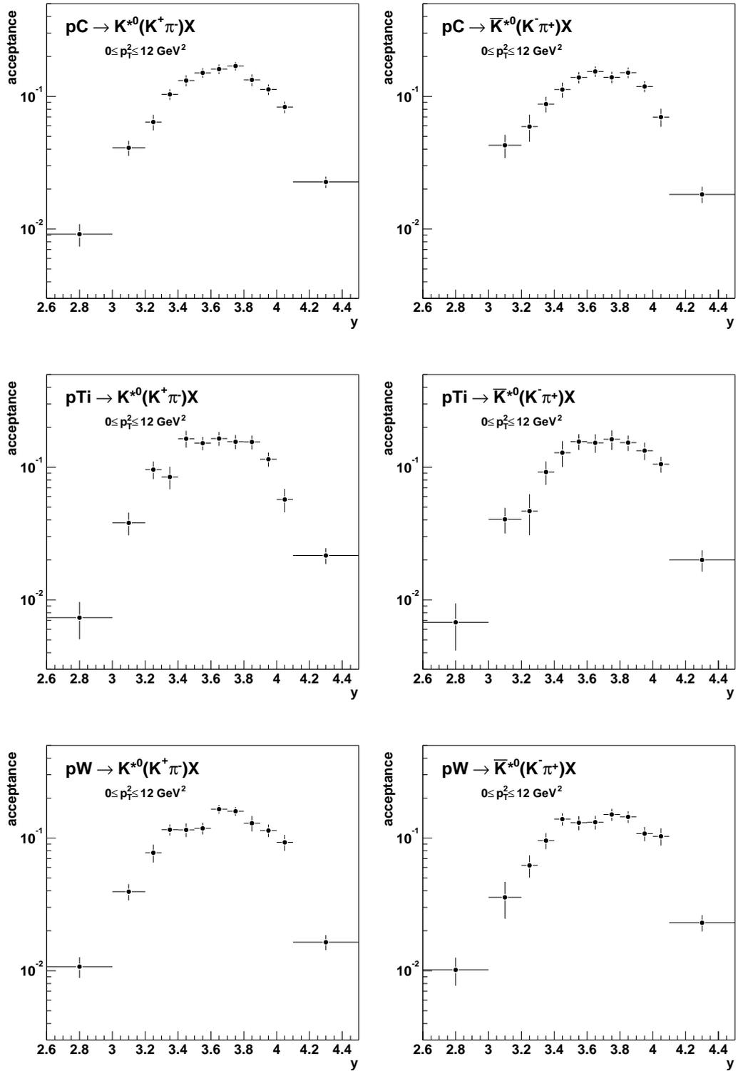
**Figure 5.18:** Acceptance in rapidity after all cuts. In the backward direction the kaon track identification limits the acceptance significantly. In the forward direction the unused Inner Tracker reduces the acceptance.
