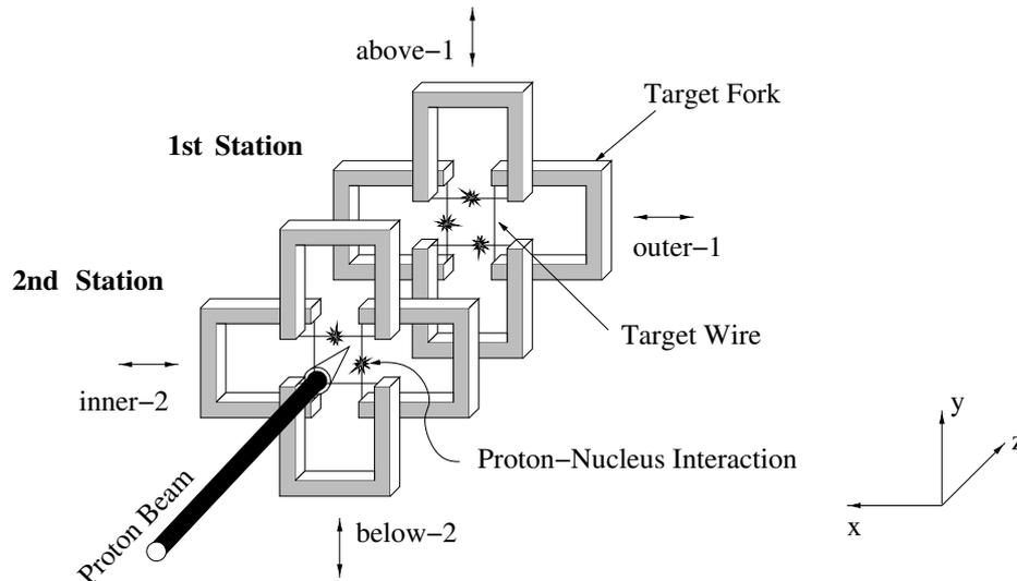
**Figure 3.5:** Sketch of the HERA-B target setup. Eight wires grouped into two stations surround the proton beam. The nomenclature of the wires is due to their position with respect to the proton beam. Based on [fun03].
