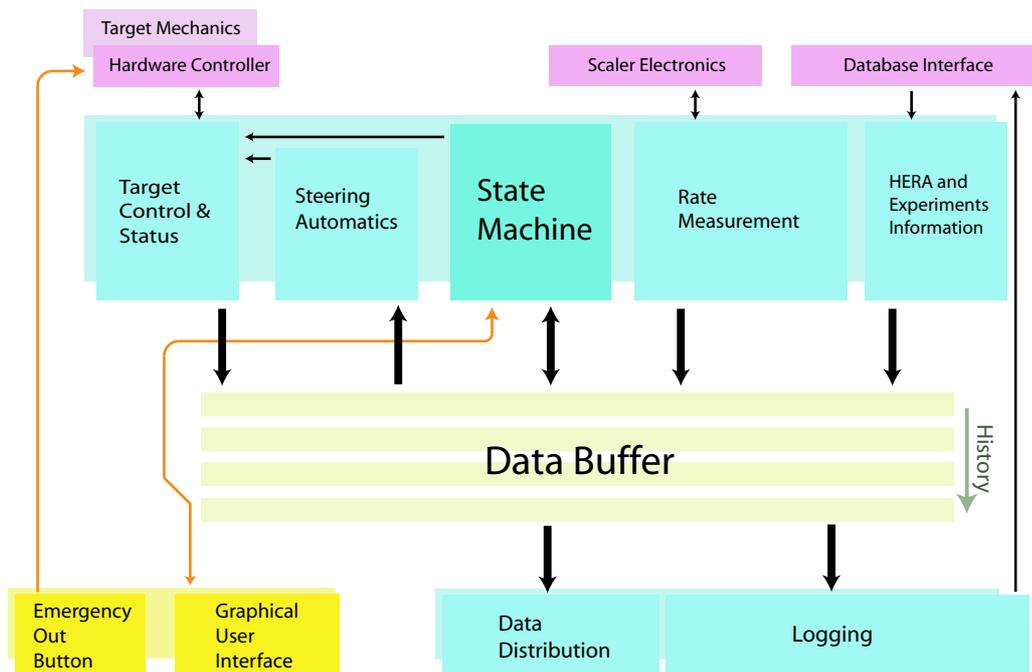
**Figure A.2:** Simplified sketch of the steering program target. The different modules (in blue) read (write) information from (to) a common data buffer. User interfaces are drawn in yellow.
