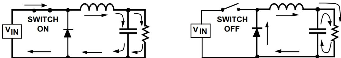
Figure 7.2: Schematic explanation of a buck converter, the arrows indicate currents [44].
