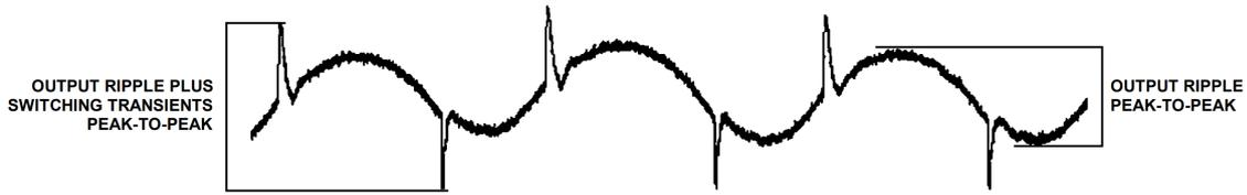
Figure 7.5: The plot shows the different between output ripple and switching transient noise [47]. In the following ripple is always output ripple plus switching transient noise.
