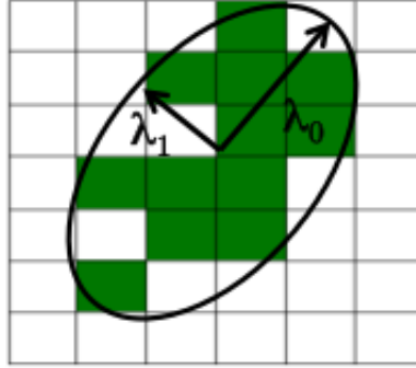
Figure 5.5: Schematic of the shower shape of a calorimeter cluster.
