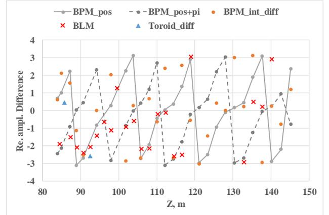
Figure 5. Comparison of phases observed in signals of BPM positions, BLMs, and differences between relative intensity signals of neighbouring BPMs. Note that  $+\pi$  and  $-\pi$  phase is the same, so that the lines on the plot connecting such points do not represent an interpolation.
