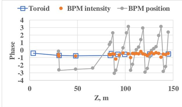
Figure 4. Phases of 0.5 Hz signal in toroids, BPM intensities and positions along the Linac.
