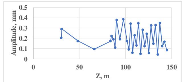
Figure 2. Oscillation amplitudes in the BPM position along the Linac. Z=0 corresponds to the ion source.
