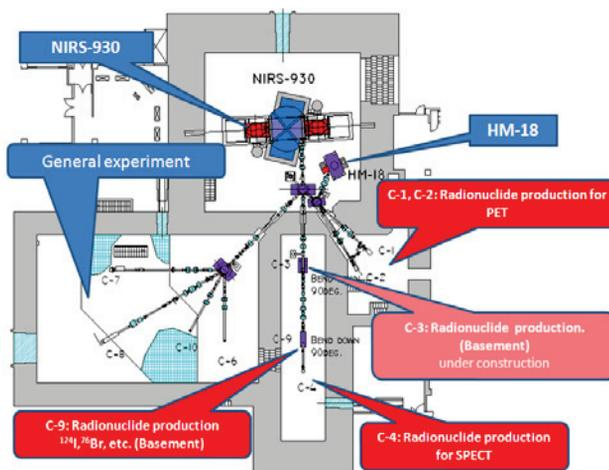
Figure 1: The system layout of the NIRS-930 facility.
