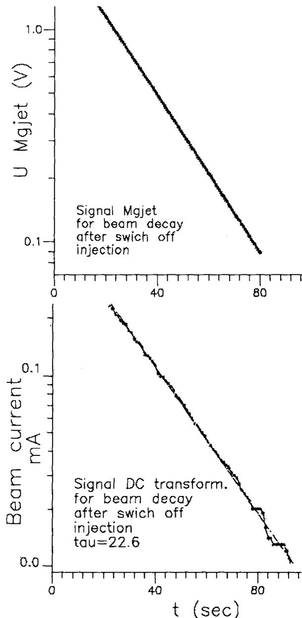
Fig.4 Two plots of decay measurements by Mg-Jet Profile Monitor and by DC transform for low beam current.
