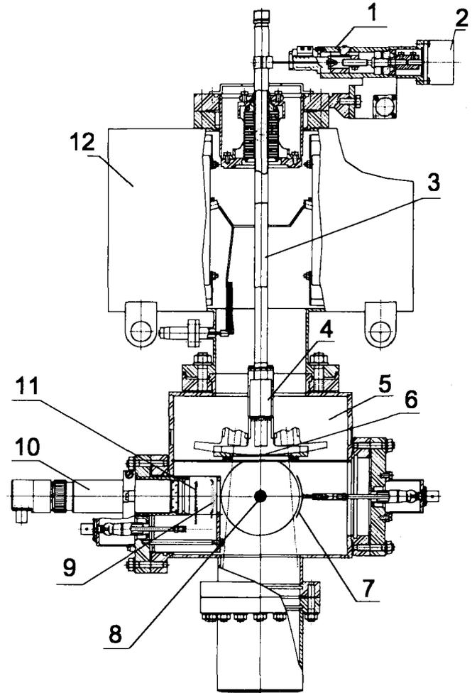
Fig. 1 Cross-section View of Magnesium Jet Profile Monitor (1-drive mechanism, 2-step motor, 3-step motor driven stem, 4-magnesium filled container with heating wires and thermocouples, 5-installation case, 6-collimator gap for outflowing magnesium jet, 7-reflecting (or clearing) electrode (under up to  $-2\text{kV}$ ), 8-beam of charged particles, 9-electrons extracting grid, 10-PMT, 11-collector plate: a glass covered with aluminized luminophor (under up to  $+15\text{kV}$ ), 12-ion pump)
