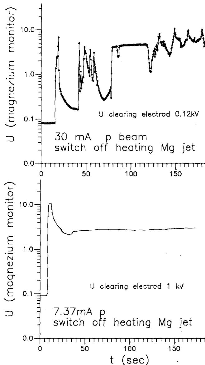
Fig.5 Signals of ionization current. Top and bottom curves are differ by cleaner electrode potential.
