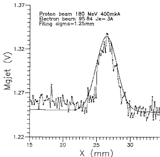
Fig. 3 Proton beam profile along X-axis obtained by Mg-Jet Profile Monitor and its fitting-curve.
