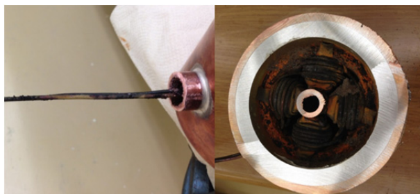
Figure 10: Enamel coating separation from the wire (left) and the yoke covered with rust (right).
