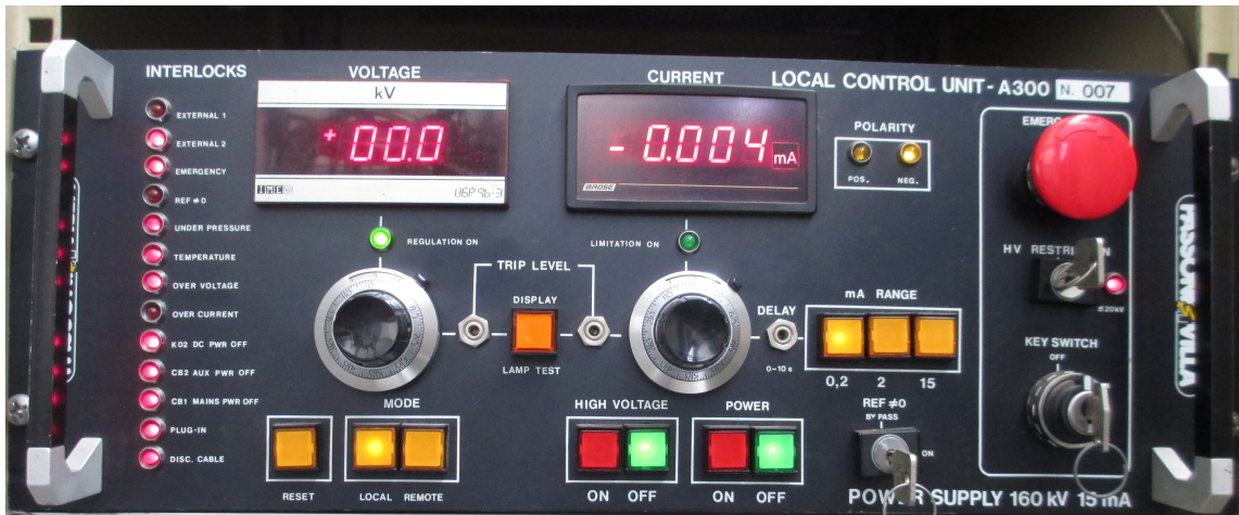
Figure 5.3: Control panel of the high voltage power supply used for testing
