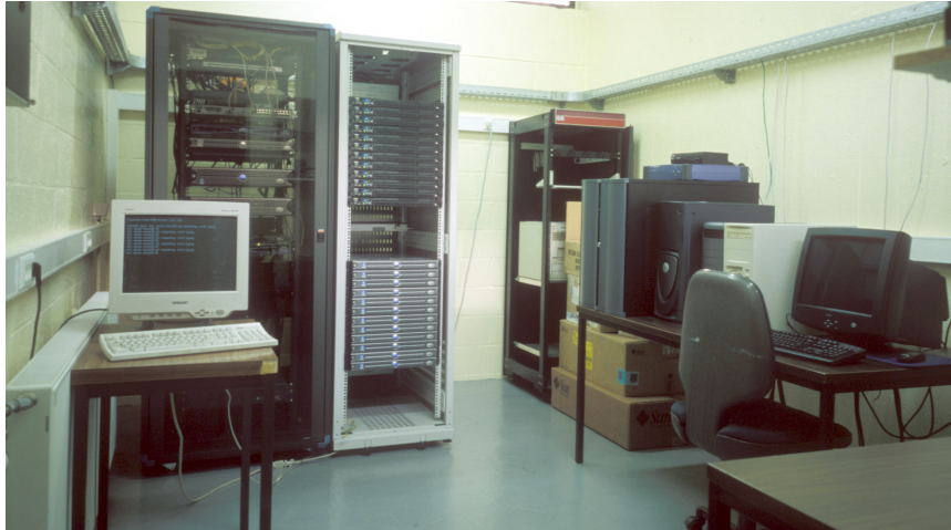
Figure B.2: Photograph of the new computer center refurbished in the context of this project. The mass storage and the software repository are placed on the table on the right, while computing nodes sits in the (opened) white rack. The second rack regroups servers of the institute, the commodity network and the link to the Internet.
